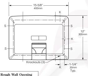
Rough Wall Opening 13-3/4" (350mm) wide 9-1/2" (240mm) high 3-3/4" (95mm) minimum recessed depth
