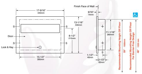
Rough Wall Opening 15-7/8" (405mm) wide 11-7/16" (290mm) high 2-3/4" (70mm) minimum recessed depth
