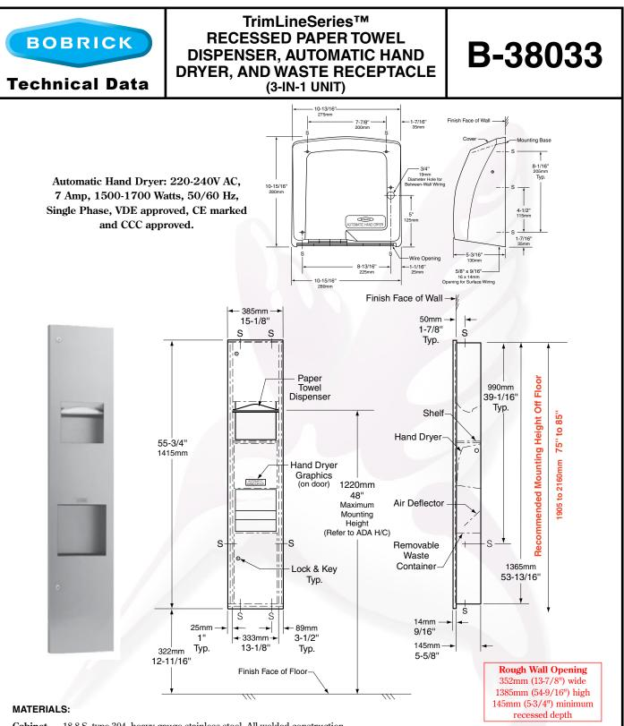
Cabinet — 18-8 S, type-304, heavy-gauge stainless steel. All-welded construction.
