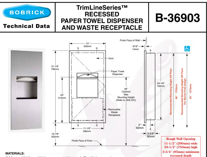
Cabinet — 18-8 S, type-304, heavy-gauge stainless steel. All-welded construction.
