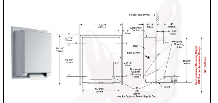
Rough Wall Opening 16" (405mm) wide 18-7/8" (480mm) high 4" (102mm) minimum recessed depth
