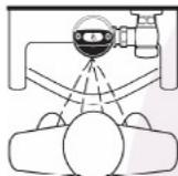
2. As the user enters the beam's effective range (15" to 30") the beam is reflected into the Scanner Window and transformed into a low voltage electrical circuit. Once activated, the Output Circuit continues in a "hold" mode for as long as the user remains within the effective range of the Sensor.
