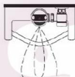
3. When the user steps away from the Sloan ECOS sensor the sensor initiates an electrical signal that operates the solenoid. This initiates the flushing cycle to flush the fixture. The circuit then automatically resets and is ready for the next user.
