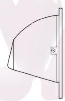
After hands are withdrawn from the Sensor's detection zone, or after a maximum of ninety (90) seconds of continuous operation, the Hand Dryer automatically stops. It is then ready for the next user.
