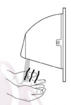
When the Infrared Sensor detects hands beneath the exhaust port, it activates the Hand Dryer. A powerful flow of warm air dries hands within thirty (30) seconds.
