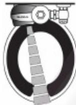
1. A continuous, invisible light beam is emitted from the OPTIMA Plus® Sensor.
