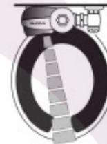
3. When the user steps away from the OPTIMA Plus® Sensor, the circuit immediately initiates an electrical "one-time" signal that operates the Solenoid. This initiates the flushing cycle to flush the fixture. The Circuit then automatically resets and is ready for the next user.
