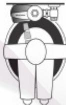
2. As the user enters the beam's effective range (15" to 30") the beam is reflected into the OPTIMA Plus® Scanner Window and transformed into a low voltage electrical circuit. Once activated, the Output Circuit continues in a "hold" mode for as long as the user remains within the effective range of the Sensor.
