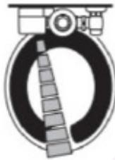
1. A continuous, invisible light beam is emitted from the Object Lock Infrared Sensor.
