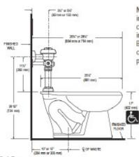
NOTE: All vitreous china dimensions shown in these drawings are nominal. Dimensions can vary within the tolerances established in the governing ASME A112.19.2/CSA B45.1 standard. Please take this into consideration when planning rough-in and plumbing layouts.
