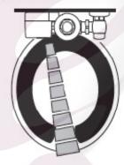
When the user steps away from the Object Lock Infrared Sensor, the circuit initiates the flushing cycle to flush the fixture.
