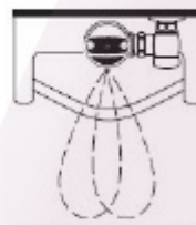
3. When the user steps away from the Sloan Solis® Sensor, the Sensor initiates an electrical signal that operates the Solenoid. This initiates the flushing cycle to flush the fixture. The circuit then automatically resets and is ready for the next user.
