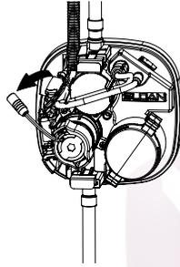
Remove new filter from control module cover.
