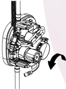
Snap new filter onto solenoid caddy assembly.
