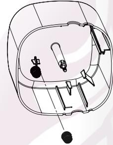
Turn solenoid caddy counterclockwise lining up arrows on control module and solenoid caddy assembly.
