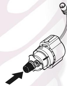
Remove solenoid caddy assembly from control module by pulling straight out.
