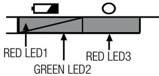
**NOTE: LED1 and LED2 are for battery and programming related items. LED3 is for solenoid service.**
