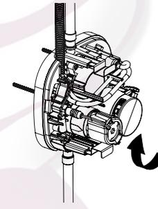
Reconnect solenoid caddy wire to control module.
