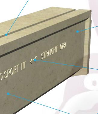
Polymer concrete - durable, yet lightweight, material made from polyester resin binder reinforced by mineral aggregates and fillers. Provides up to four times the compressive strength of cement concrete and almost twice the compressive strength of HDPE. Offers a thermal expansion ratio similar to the concrete surround, particularly important where long runs are used to prevent 'buckling.'
