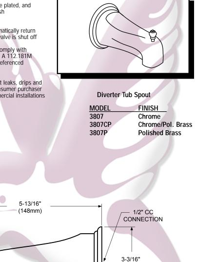
(81mm) 1-1/8" (29mm) Finished Wall Line CRITICAL DIMENSIONS (DO NOT SCALE)
