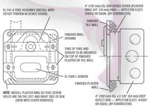
To ensure a perfect rough-in, Sloan recommends the use of the EL-485-A Flushometer Electrical Box Positioning and Support Kit. Specify and order the EL 485-A Kit separately. Consult factory for installation details.
