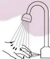
3. When hands are moved away from the Optima Sensor, the loss of reflected light initiates an electrical signal that deactivates the solenoid valve, shutting off the water flow. The circuit then automatically resets and is ready for the next user.
