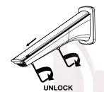
Rotate solenoid assembly counterclockwise through a 45° angle.
