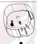
Turn solenoid caddycounterclockwise lining up arrows on control module and solenoid caddy assembly.
