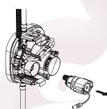
Insert solenoid caddy assembly into control module lining up arrows. Turn solenoid caddy assembly clockwise 45°.
