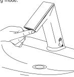
Cover IR clic until LED flashes 4x - hold on until LED flashes 1x to 8x, from minimum to maximum. See diagram below. Release when requested range is reached.
